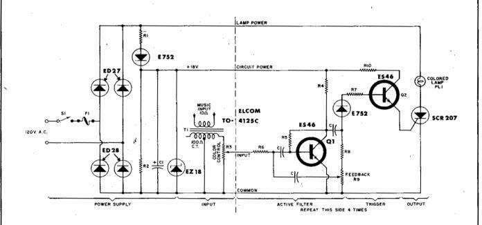
R1-1500 ohm, 10 W res. ±10% R2-820 ohm, 1 W res. ±10% R3-50 ohm por "Color Control" C1-15 μF, 35 V elec. capacitor S1-10 A toggle sw. F1-10 A, 120 V fuse
